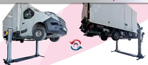
Symmetric lifting arms means vehicles can be loaded in either direction, making it much more versatile.
