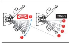
Our locking mechanism, via spindle as opposed to the cog style, allows for far greater choice of positioning for the operator.
