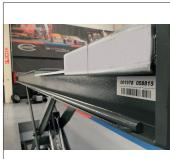
Includes sliding guide for Jacking Beams.
